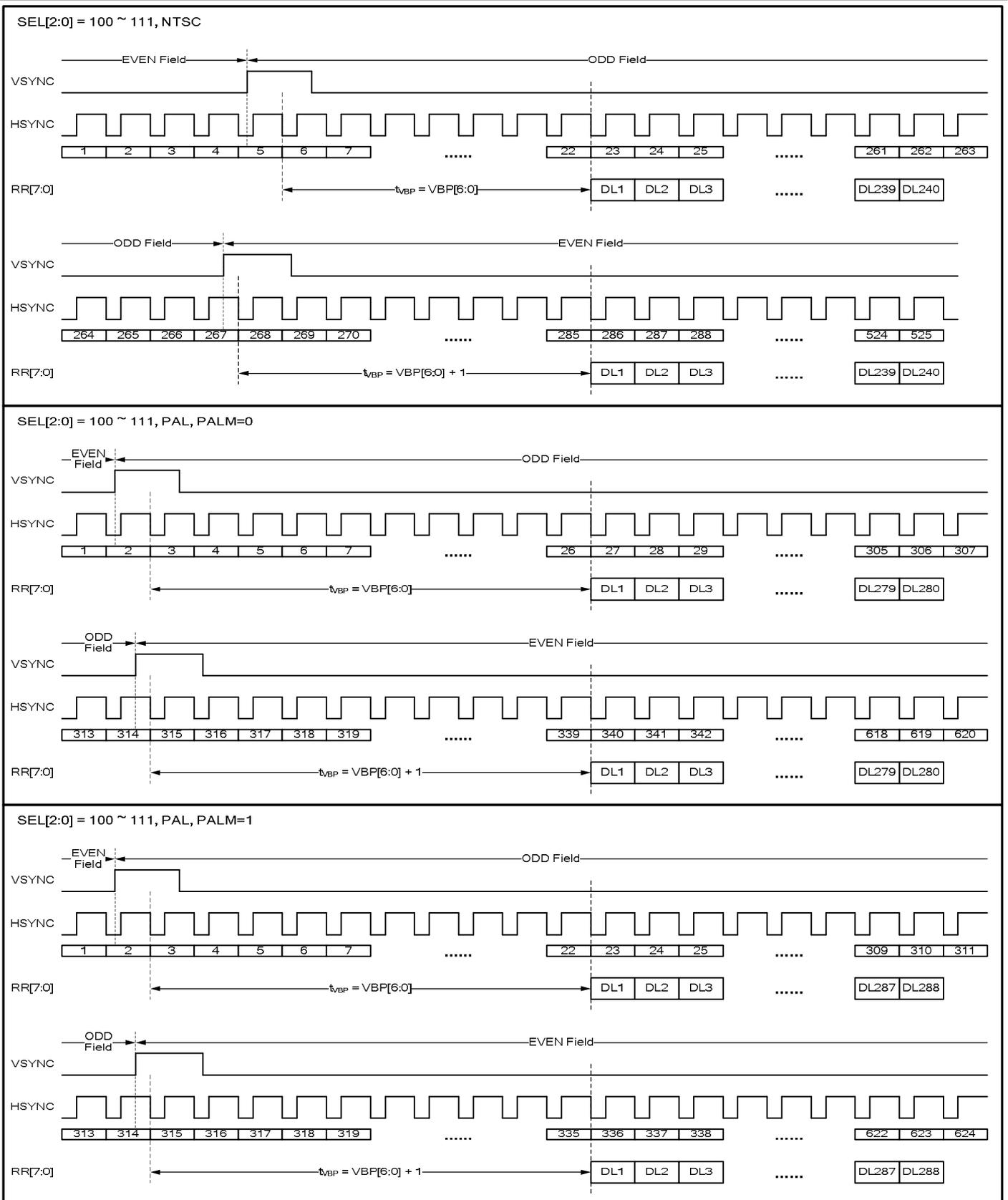
Figure 1 CCIR601 Vertical Timing
