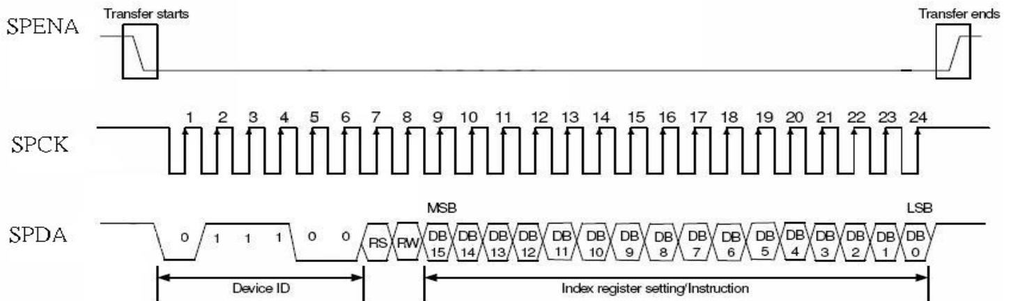
**Figure 9 SPI timing**
